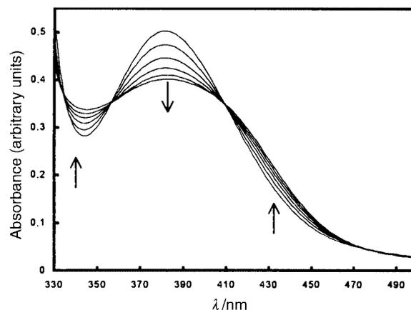
Fig. 4 Spectral changes observed during the isomerization reaction **4a** → **4b**; CHCl<sub>3</sub>, 25 °C, [Pd<sup>II</sup>]<sub>T</sub> = 0.002 M.
